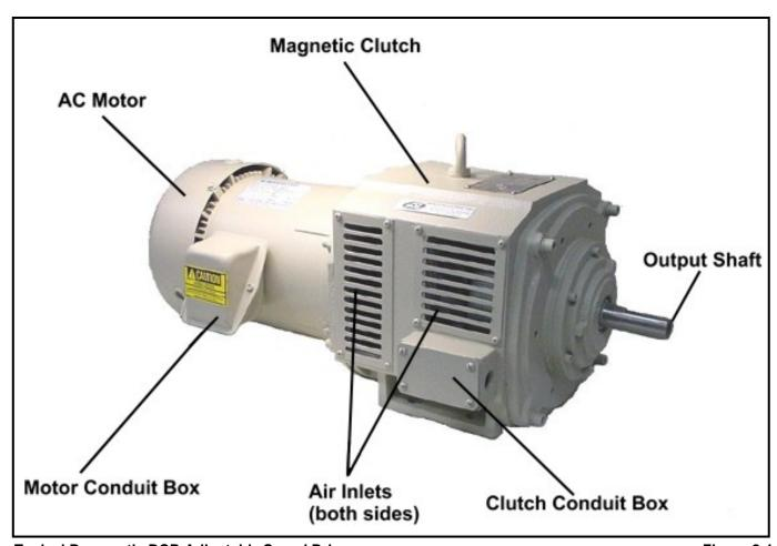
Typical Dynamatic DCD Adjustable Speed Drive
