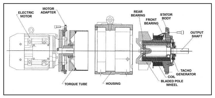
**Typical Assembly Drawing of DCD Drive**
