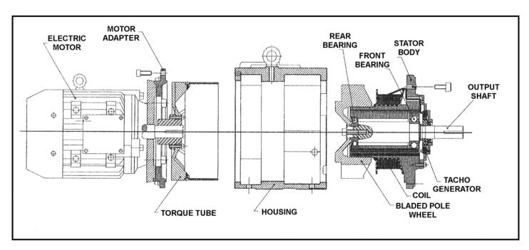
**Typical Assembly Drawing of DCD Drive**
