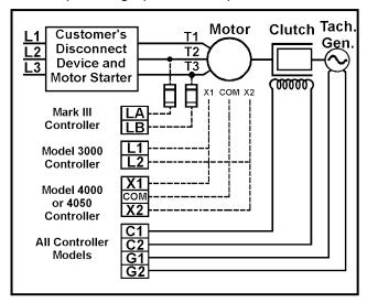
**Typical Wiring Connections**
