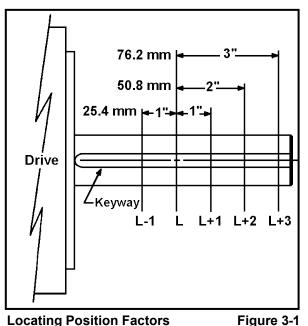
Generally, the device should be installed on the shafts by following the device manufacturer's instructions. Devices with split hubs or light interference fits that use
