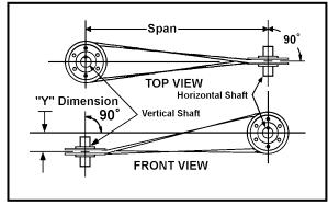
**Perpendicular Shaft Alignment**
