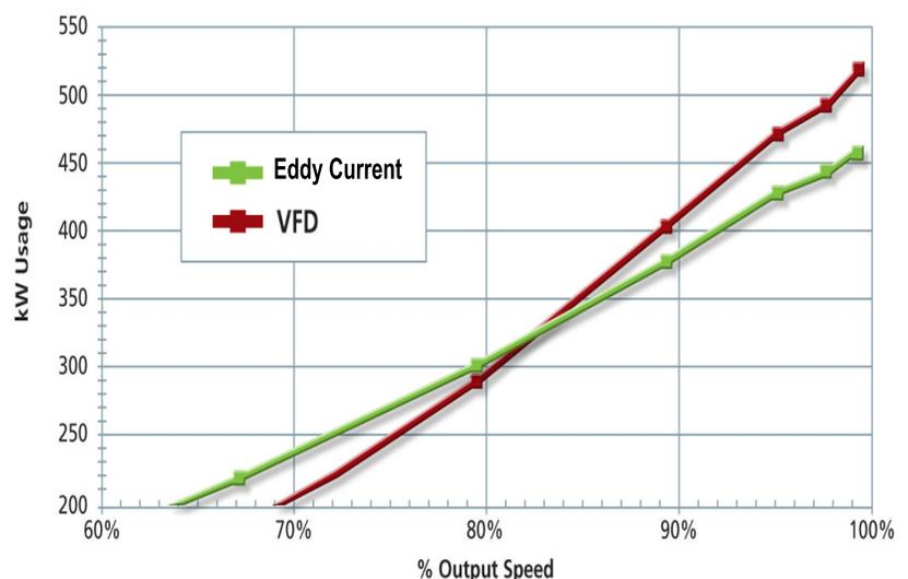
**Figure 2:** This pump operates from minimum flow at 80% speed to full flow at 100% speed
